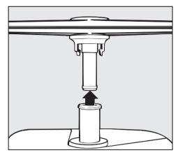
■ Pull the <u>lower</u> spray arm firmly upwards to remove it.
